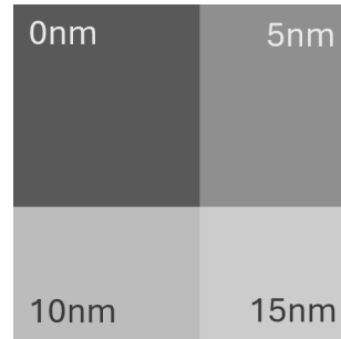
Figure 3.12: Scheme of deposition of silver layer: in order to obtain three distinct silver thicknesses, two successive depositions were performed. The first deposition consisted of 5nm, applied while masking half of the sample. The second deposition of 10nm, was carried out after rotating the mask by 90^\circ . With this procedure four quadrants with different thicknesses, including one without any silver, were obtained.
