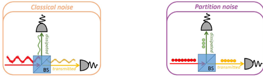
Figure 1.3: every beam exiting from a beam splitter presents two noise contributions: a classical one, related to the beam intensity, and a quantum one, determined by the random division of photons that occurs on the beam splitter.
